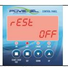
In cases of shutdown and subsequent restart, the rectifier is in the shutdown state. It is possible, however, to set the rectifier so that when it is turned back on it is in the state prior to being turned off (if off it stays off, if on it restarts but without ramping.
