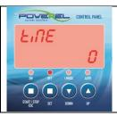
In case of end cycle mode **On** active, with this function iis possible to set the time of notification signal.
